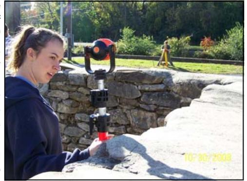
Unit 3 in the annex of the dye works, students using the Total Station to "shoot out" the coordinates for later 3-D graphics
